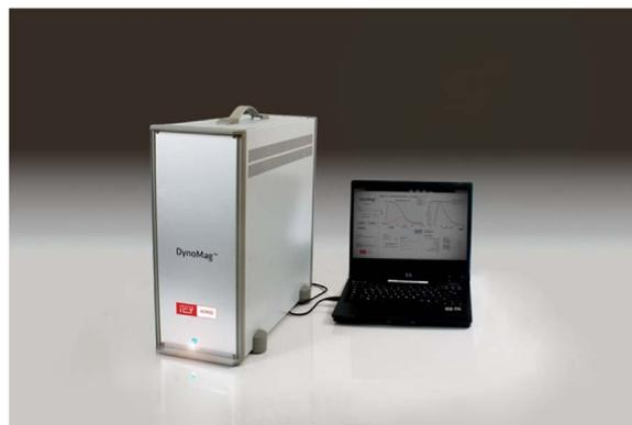
Fig. 1. The figure shows the Acreo DynoMag system including the integrated electronics with the coil system (excitation and detection, inside the aluminum box) and the dedicated software that controls the measurement and performs the magnetic analysis.
