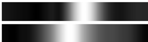
Fig. 9. Phantom image of two adjacent lines/dashes, one filled with a FeraSpin™ XL suspension ( \eta_1 , top) and the other with the same particles immobilized in a Mannitol-D matrix ( \eta_2 , bottom).
