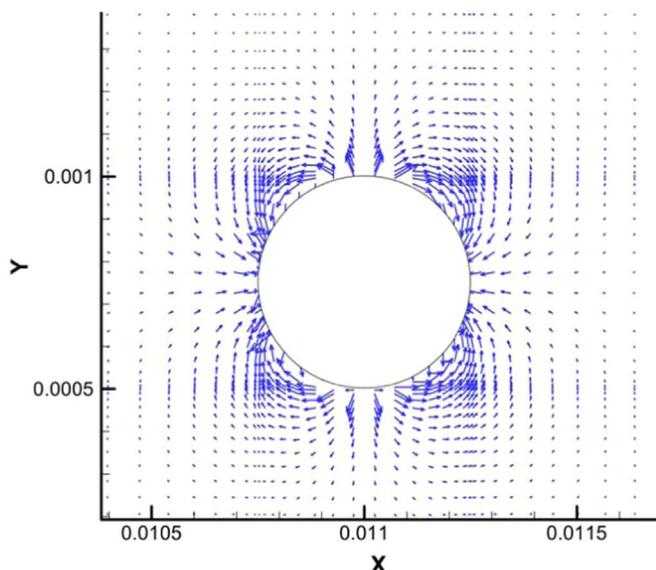
**Fig. 1.** Schematic drawing of the spatial distribution of the magnetic force acting on magnetic particles in the vicinity of a magnetic filter wire in magnetic fields. White large circle represents the cross section of the magnetic wire. The magnetic field applied in a horizontal direction. The direction and the length of arrows correspond to the direction and the intensity of the magnetic force.
