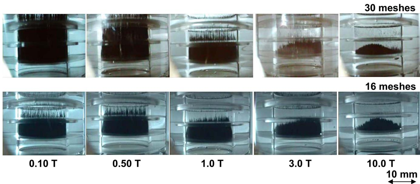
Fig. 7. Dependence of particle deposition on applied magnetic fields. Upper column: in case of the magnetic filter of 30 meshes, lower column: 16 meshes.
