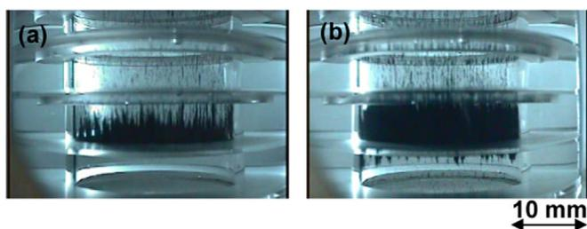
**Fig. 5.** Examples of particle deposition process. The sample suspension was flowed with the speed of 2.5 ml/s (a) and 19 ml/s (b), using a magnetic filter of 16 meshes under 0.1 T.
