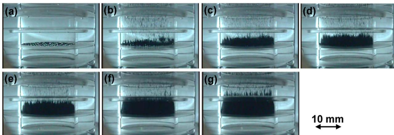
**Fig. 4.** Observed deposition process of magnetic particles. The sample suspension was flowed with the speed of 8.4 ml/s using a filter of 16 meshes under 0.50 T. beginning, (b) after 20 s, (c) 30 s, (d) 40 s, (e) 50 s, (f) 90 s, (g) 120 s.
