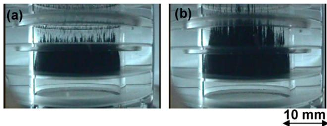
**Fig. 6.** Dependence of spike length on the flow rate. Both of them were observed under 0.50 T using a filter of 16 meshes. The flow rates of the sample suspension were 8.4 ml/s (a) and 2.9 ml/s (b), respectively.
