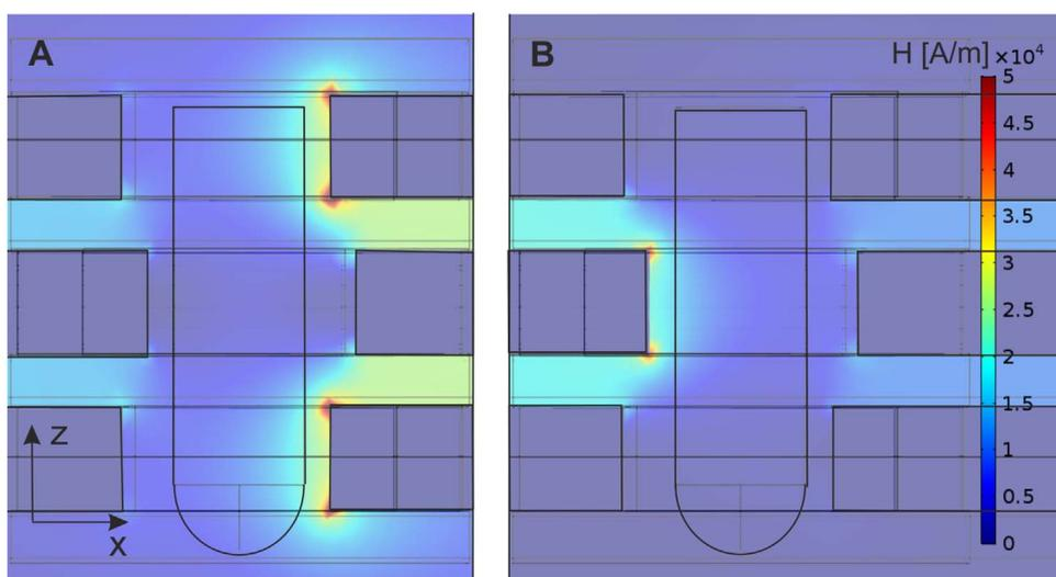
**Fig. 9.** Side view of the magnetic fields obtained from the simulation in the ESM with three magnetic planes and a current of 400 mA. A: process step 1 (upper and lower magnets are charged) with two coils. B: process step 2 (middle magnet is charged) with one coil.
