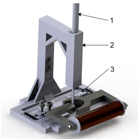
**Fig. 3.** CAD illustration of the setup for magnetic induction  $B$  measurements, 1: magnetometer; 2: gallows; 3: base plate with slide system.
