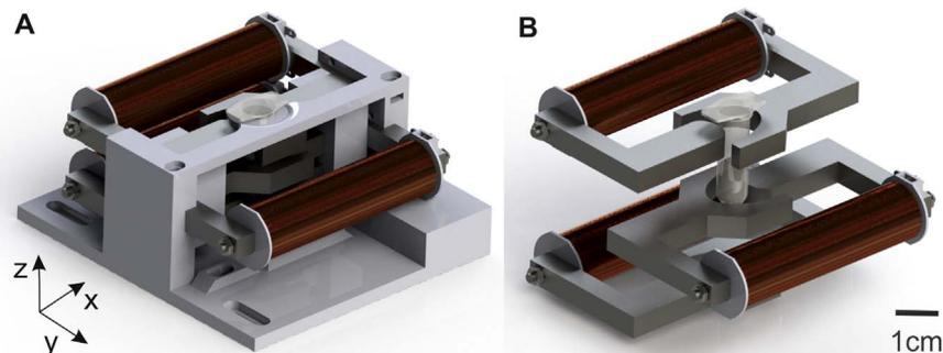
Fig. 1. CAD illustration of the ESM with three magnetic cores arranged in three planes, where the middle plane has the opposite direction of elliptical pole shoe geometry which can be seen in A: in the 3D printed holder to fix the positions of the magnetic cores, and in B: exploded view of the three planes of magnets.
