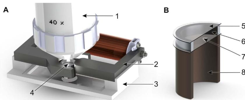
**Fig. 2.** CAD illustration of the setup for microscopic imaging of SMP movement. 1: long working distance lens; 2: magnetic core with coil; 3: holder; 4: fluid chamber seen in B, 5 and 7: cover slips to close the chamber 6; 8: spacer.
