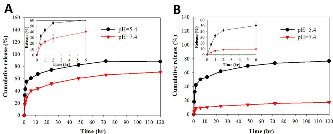
Fig. 5. The pH-dependent drug release profile of CPT-11 (A) and DOX (B) from mGOC-PEG.
