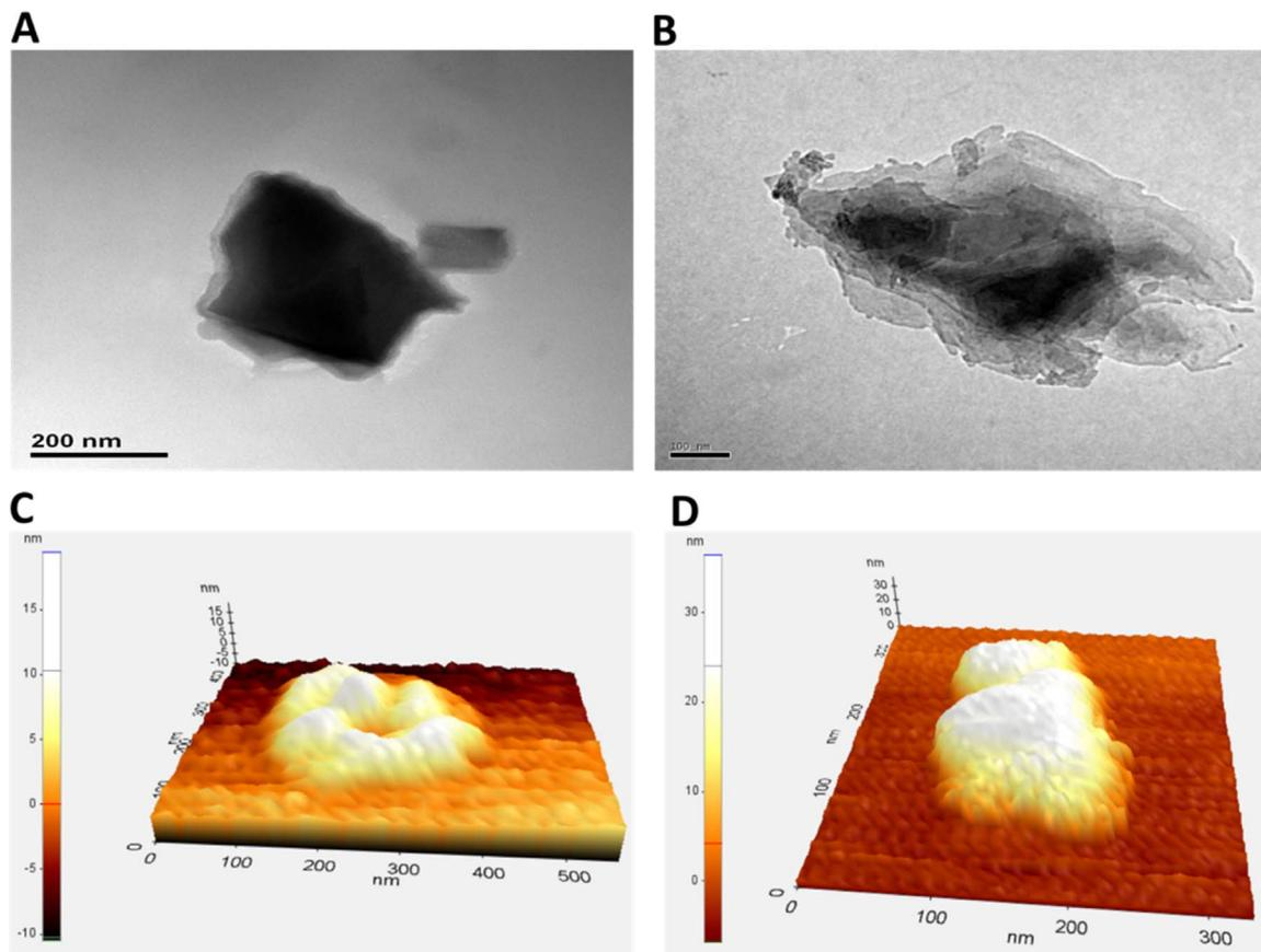
Fig. 1. TEM images of (A) GO (bar=200 nm) and (B) mGO (bar=100 nm). AFM images of (C) mGO and (D) mGOC.
