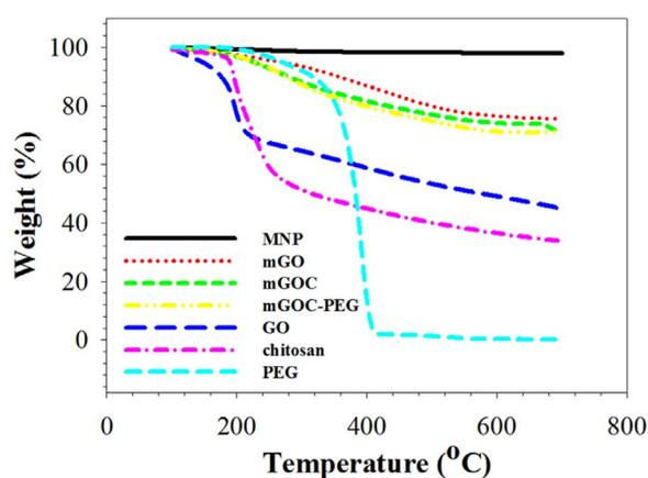
Fig. 3. Thermogravimetric analysis (TGA) of nanocarriers and polymers.
