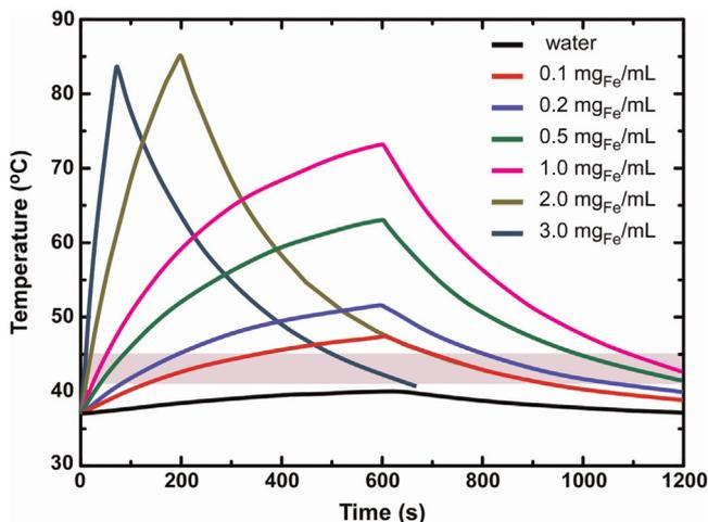
Fig. 2. Time dependent temperature curves for sample FluidMAG-DX-100 nm, for various concentrations (0.1–3 mg<sub>Fe</sub>/mL), under 24 k A/m field amplitude. Shaded band denotes the desired hyperthermia levels.
