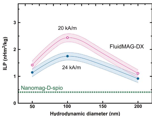
**Fig. 4.** ILP values (presented as shaded bands including the error bars) for samples FluidMAG-DX-50, 100, 200 nm, measured in concentration 1 mg<sub>Fe</sub>/mL, under 765 kHz and 20, 24 kA/m. The dotted line corresponds to Nanomag<sup>®</sup>-D Spio.
