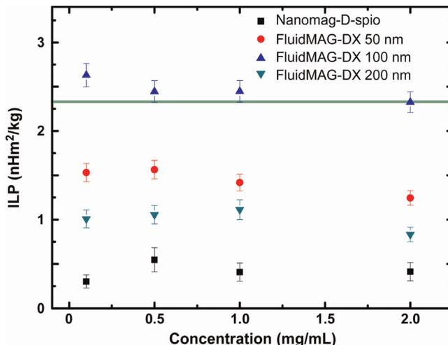
Fig. 3. ILP values vs. concentration, under 20 kA/m field amplitude. Reference line refers to sample FluidMAG-D from Ref. 10.
