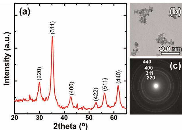
Fig. 1. Structural characterization schemes: XRD pattern (a) and TEM image (b) along with the EDP (c) for sample FluidMAG-DX-100 nm.
