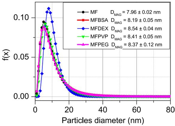
Fig. 5. Comparison of the core particle diameter obtained by fitting of MFs magnetization curves.
