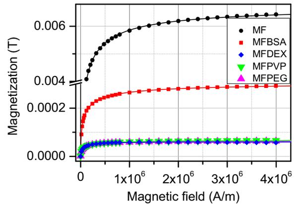
Fig. 4. Magnetization curves of MFs measured at room temperature.
