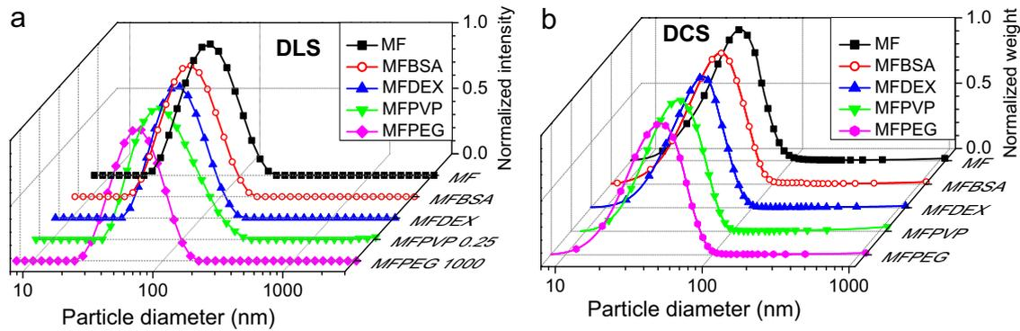
Fig. 3. Comparison of the particle size distributions of MFs determined by DLS (a) and DCS (b) method.
