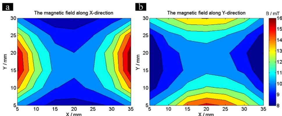
**Fig. 2.** The distribution of the static magnetic field flux density in each orientation. (a) the measurement of magnetic field along X-direction, and (b) the measurement value along Y-direction. The uniform area is about 12 mm x 10 mm with the error less than 10%.
