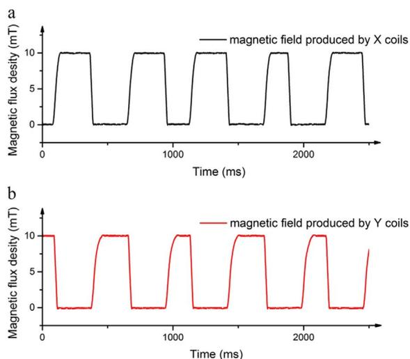
**Fig. 3.** The waveform of the swing magnetic field. (a) the magnetic flux density along the X-direction, (b) the magnetic flux density along Y-direction. The rise time is about 100 ms and fall time about 60 ms.
