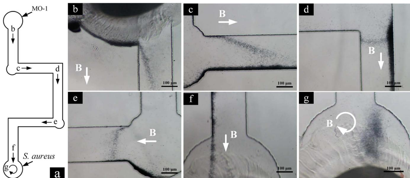
**Fig. 4.** The movement of MO-1 under applied magnetic fields in a microfluidic chip. (a) the microfluidic chip. (b)–(f) illustrate the targeted move of MO-1 under gMF, swimming along the magnetic field direction and turning around as the direction changed, and (g) presents the rotation of MO-1 under rMF.
