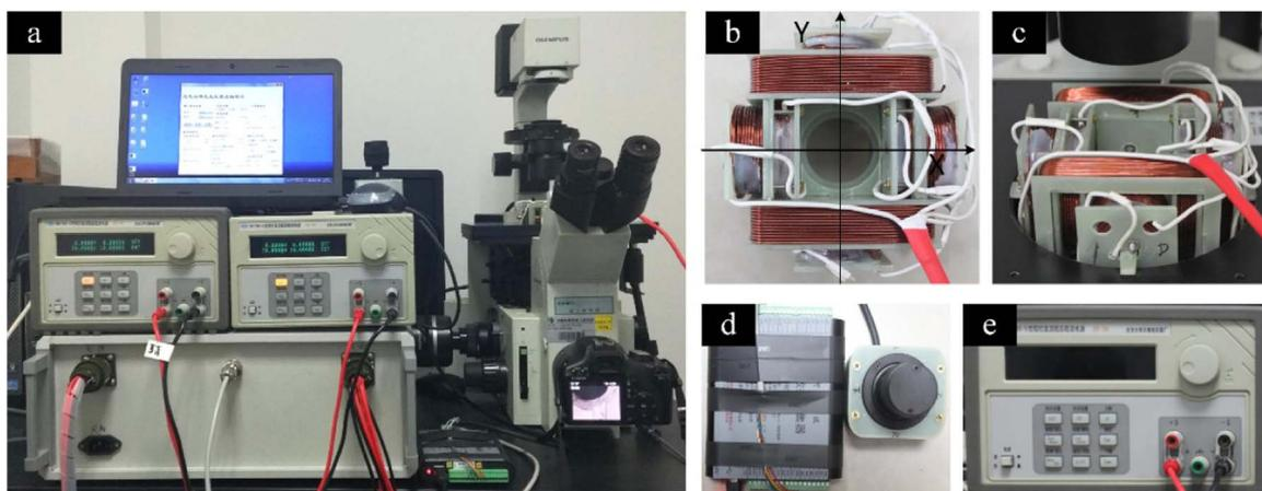
**Fig. 1.** The compound magnetic field system. (a) the compound system, (b) the coils, (c) coils device embedded into microscope platform, (d) the handle joystick connected with a DAQ device, (e) the power supply panel.
