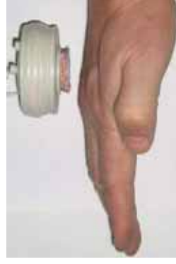
Fig.1. The coil system detects MP on the other side of the hand
